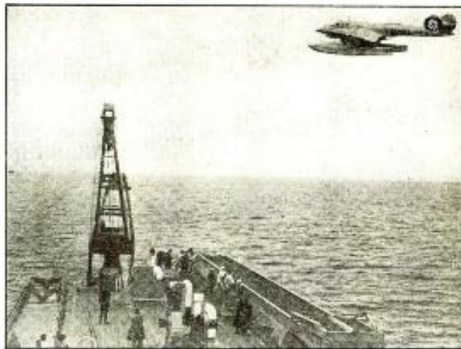
The deck of the first airplane-hotel ship, with large crane for raising plane from water. Note the catapult at the right.
